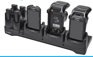
Requires Power Supply (PWR-BGA12V108W0WW), DC Line Cord (CBL-DC-382A1-01 or CBL-DC-381A1-01), and Country Specific Line Cord.
